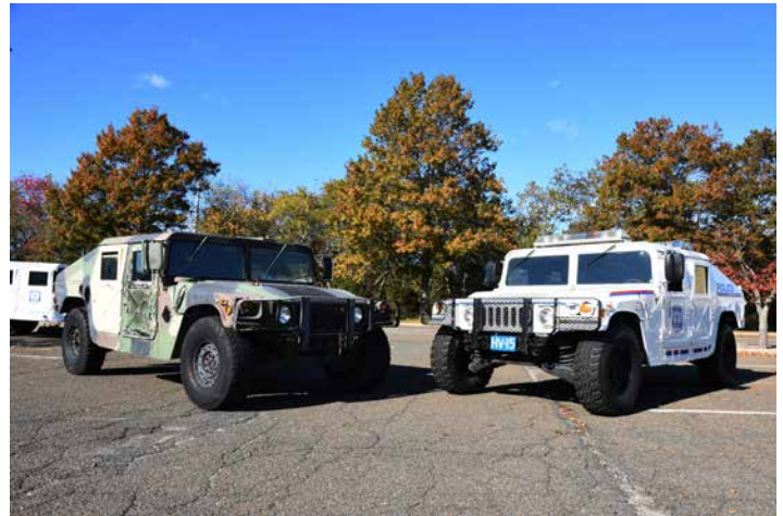
Before and after - the contrast between the military version of the Humvee and one that was repurposed for civilian law enforcement usage. All the mounting brackets were removed, the turret was removed, and the vehicle was painted to match other vehicles in the department's fleet.
