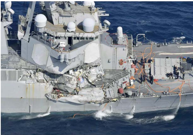
The damage of the right side of the USS Fitzgerald. AP
