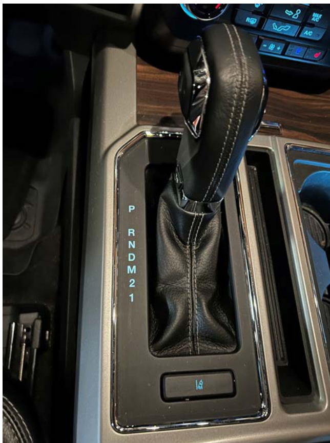
F150 – An example of a mechanically linked shifter.
