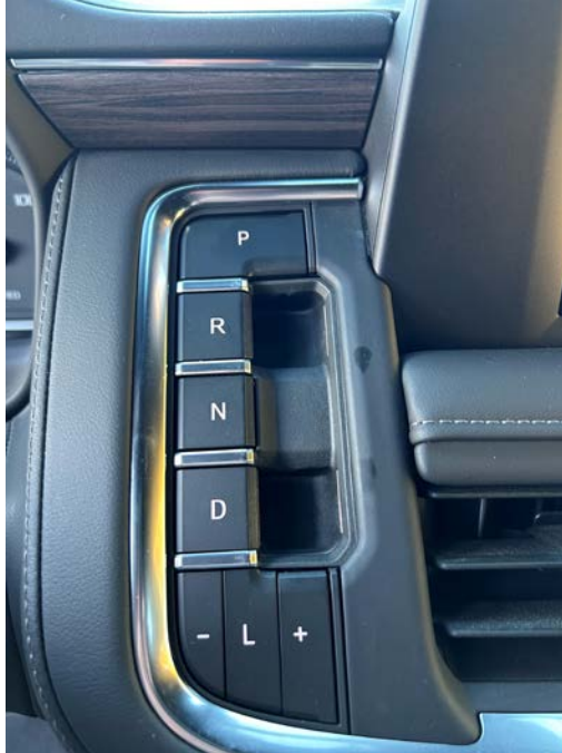
Tahoe – A push / pull style computer-controlled transmission selector
