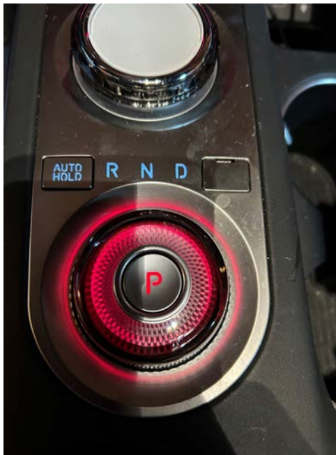
Genesis – A rotary computer-controlled transmission selector.
