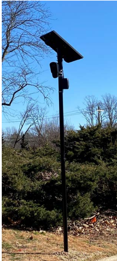
Solar powered ALPRs with LTE capability can easily be deployed anywhere with sufficient sunlight.
