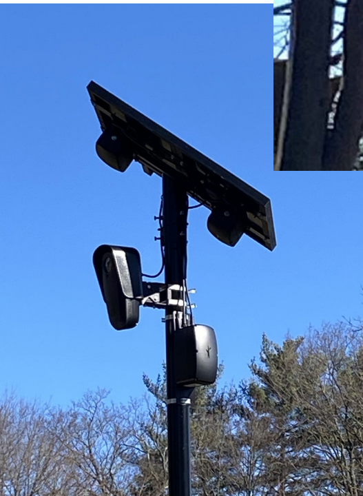
Fixed LPR / Fixed LPR2 / Mobile LPR - License plate readers, whether fixed or mobile, can be a cornerstone technology in RTCCs, constantly monitoring for wanted and stolen vehicles.
