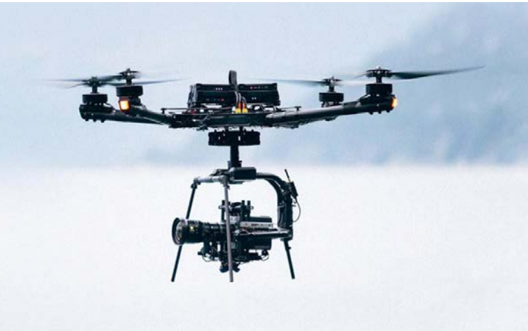
The Alta X has a payload capacity exceeding 35 pounds.
